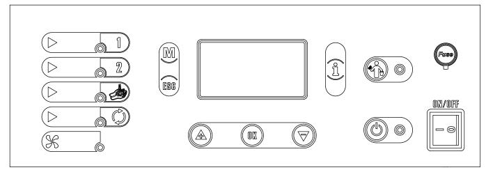
The control panel is managed by a microprocessor. The temperature detection system uses thermocouples. The large display improves the appliance management by making read-outs and functions promptly available. The various control buttons are described below.
