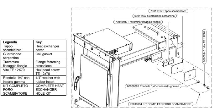
6) Insert the safety heat exchanger inside the appliance as illustrated in the following figure. Then remount the COMPLETE HEAT EXCHANGER HOLE KIT and tighten screw 60006245 all the way.
