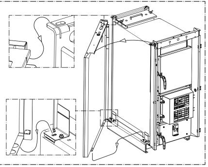
4) Undo screw 60005227 completely and screw 60007780 only partially Attention: Only partially undo screw 60007780 to prevent the coil fastening plate from falling inside the body of the appliance!
