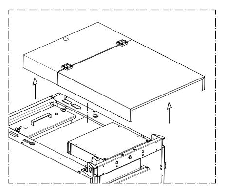
2) Undo the two M10 wing nuts on the complete inspection door and remove it by pulling upwards. Next, remove the rivet 8X35 and remove the whole spiral tube scraper lever by pulling it outwards:
