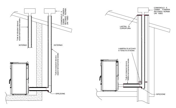
The user must possess a certificate of conformance for the flue outlet (Ministerial Decree 22 January 2008, no. 37). The flue outlet must be built in compliance with UNI 10683.
