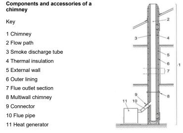
ATTENTION: wall outlets, that is outlets installed on the outer front wall without the use of a chimney/flue outlet /flue pipe to convey the combustion products to the roof, are strictly prohibited.
