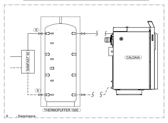
**ATTENTION:** before loading the system, it is mandatory to verify that the preload pressure of the expansion tank or expansion tanks is 1.5 bar. Next load the system until it reaches a pressure of 1 bar.
