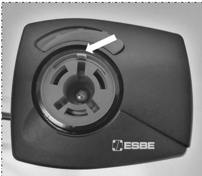
**5** – Attach the motor to the valve using the Philips head screw provided. Always make sure the position of the rotor and the green tooth are as shown in the picture above.
