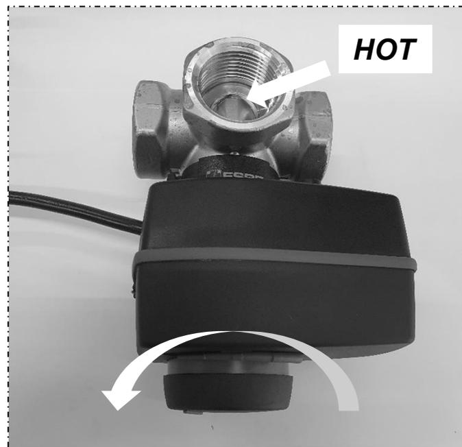
**7** – To check whether the installation has been successful, rotate the extracted cap anti-clockwise until the end stop. If the HOT branch is completely closed, then the installation was successful, otherwise start the procedure again.
