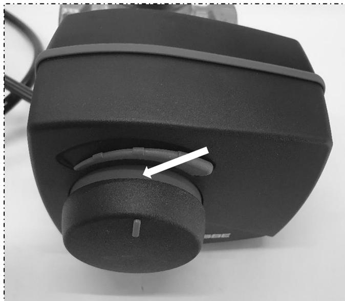
**6** – Insert the cap removed until the end stop by pushing it towards the motor. Afterwards, pull the same cap outwards until you hear a click and the red band is visible, see picture above.
