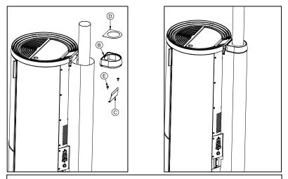
4) Fix the bracket (C) using the two screws (E) and then insert the ceramic (B) and the non-structural profile (D).
