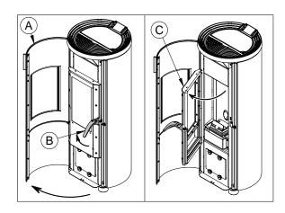
To open and close the firebox door (C) open the external door (A) and using the appropriate handle (B), release the fastening hook. At the end of this operation, it is recommended to remove the handle in order to avoid opening the door accidentally. Open the door only for cleaning operations and exclusively with the appliance cooled off and disconnected from electric power.
