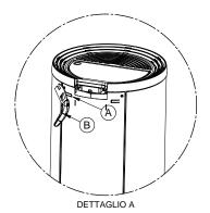
Your appliance is supplied with a handle (B) to open and close the firebox door and thus proceed with cleaning operations. When not in use, the handle can be stowed on the rear of the appliance.
