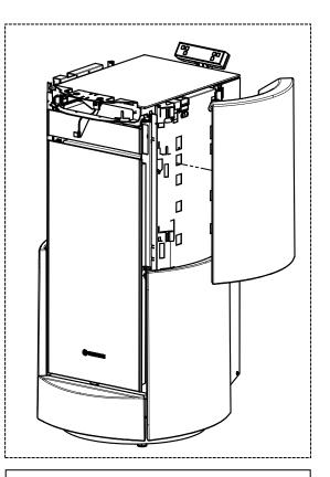
6 - Insert the upper side panel (C) on the teeth provided, as in the previous point. Slightly bend the teeth so as to firmly secure the majolica to the body. Carry out the same procedure on the opposite side.
