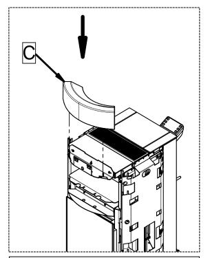
3 - Insert the upper majolica (C) on the teeth provided. Slightly bend the teeth so as to firmly secure the majolica to the body.
