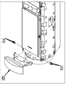
1 - Undo the 4 screws (2) and remove the majolica support bracket. Insert the lower majolica (B) on the bracket that you have just removed. Lastly fasten the bracket with the majolica using the 4 screws (2) just removed.
