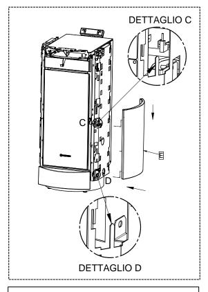
5 - Insert the lower side panel (E) on the teeth provided, as illustrated in details C and D. Slightly bend the teeth so as to firmly secure the majolica to the body. Carry out the same procedure on the opposite side.
