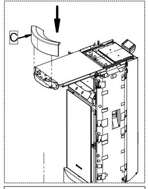
$2\,$  - Remove the tray and insert the upper majolica (C) on the teeth provided. Slightly bend the teeth so as to firmly secure the majolica to the body.
