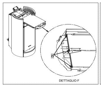
7 – Remove the pellet loading tray and loosen the 3 screws (8) underneath as shown in the detail (F). **ATTENTION:** if your appliance has a **NATURAL** body, do not carry out this operation; start directly from point 9.
