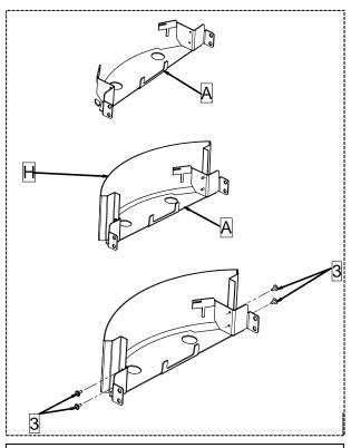
$2-{\rm Fix}$  the calendered profile (H) with the 4 screws (3) provided in the kit on the lower bracket (2 - A) just removed.
