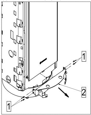
1- Undo the 4 screws (1) and remove the lower bracket (2) present on the appliance.
