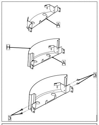
$2-{\sf Fix}$  the calendered profile (H) to the lower bracket (2 - A) with the 4 screws (3) provided in the kit.
