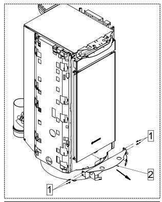
1 – Undo the 4 screws (1) and remove the lower bracket (2) present on the appliance.
