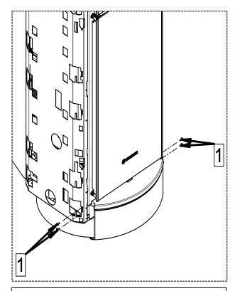
4 - Fix the assembly just created to the appliance using the previously removed screws (1).
