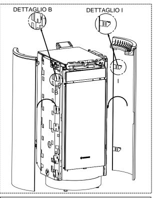
$5-{\rm Fix}$  the upper side cast iron element (F) to the side panel (C) with the screws (6) and washers (7) provided in the kit. Carry out the same operation on the opposite side.
