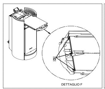
7 – Remove the pellet loading tray and loosen the 3 screws (8) underneath as shown in the detail. **ATTENTION:** if your appliance has a **NATURAL** body, do not carry out this operation; start directly from point 9.
