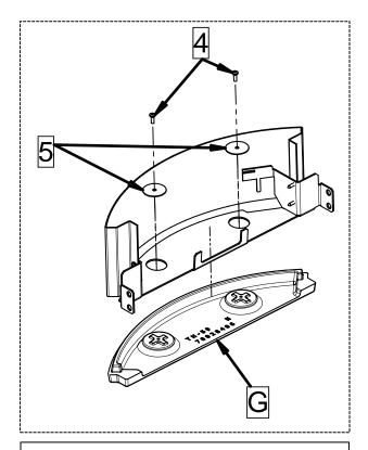
3- Fix the lower cast iron element (G) to the lower bracket (2 - A) just assembled, using the 2 screws (4) and the 2 washers (5).
